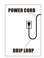
connector if an extension cord is used to prevent water travelling along the cord and coming in contact with the receptacle. If the plug or receptacle does get wet, do not unplug the cord. Disconnect the fuse or circuit breaker that supplies power to the appliance. Then unplug and examine for presence of water in receptacle.
