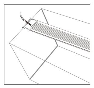
C. For maximum LED performance, it is recommended that the fixture be cleaned on a weekly basis. Unplug transformer prior to cleaning the light fixture and remove from aquarium. Use both hands when manipulating this appliance. Wipe exposed surfaces carefully with a damp cloth to remove any dust or mineral deposits that may collect over time. Do not use detergents or harsh cleaners as it can damage the light fixture.
